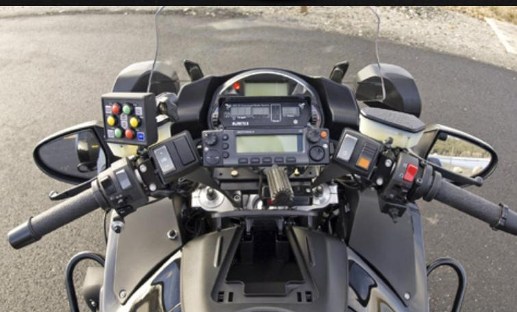
*With its standard high-output alternator, tighter turn radius, dedicated wiring harnesses and separate battery for all add-on police equipment, the Concours 14 ABS Police motorcycle supports most equipment packages specified by purchasing agencies.*
